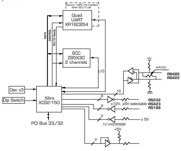
FIGURE 1 PMC-SERIAL BLOCK DIAGRAM Other configurations are built into the board layout, including a second quad UART replacing the SSC, and RS-485 I/O. Different oscillators can be
