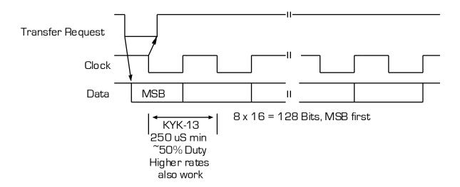
The Transfer request signal is asserted when the software accesses the "trans" address with a write. Transfer Request remains asserted until the KYK-13 responds with the clock going low. Data changes on the rising edge and is captured by the IP-Crypto on the falling edge. The KYK-13 asserts data with inverted definitions. The IP-CRYPTO
