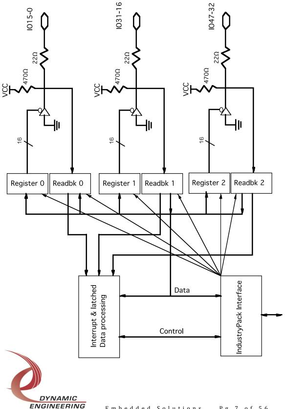
IP-Parallel-IO is part of the IP Module family of modular I/O components. IP-Parallel-IO is capable of providing multiple protocols. The TTL version provides 48 uncommitted IO. Each channel can be programmed to be input, output and interrupter. The 485 version has 24 differential pairs. TTL and Differential pairs can be mixed to have any combination of TTL and Differential IO. Please refer to the ordering table to see the standard IO options.
