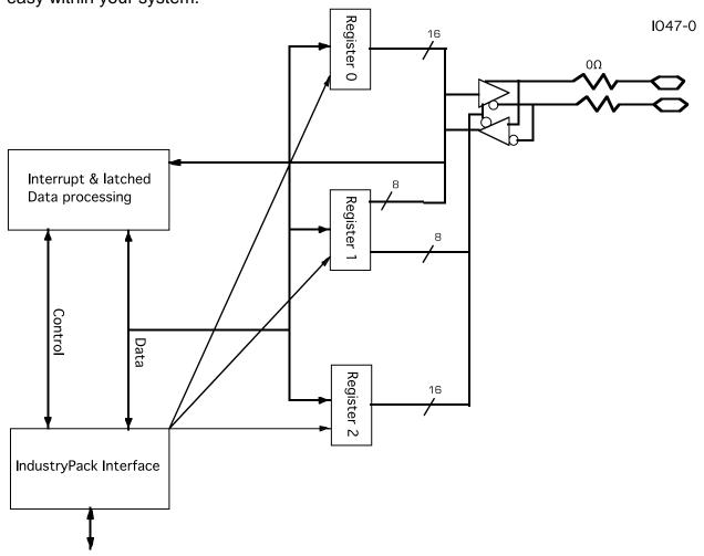
In the versions with 485 transceivers the control bits have an alternate definition. The bits are paired; one the direction control and one the data bit. In the TTL version, all of the bits are data bits. Please refer to the diagram of the -485 version.
