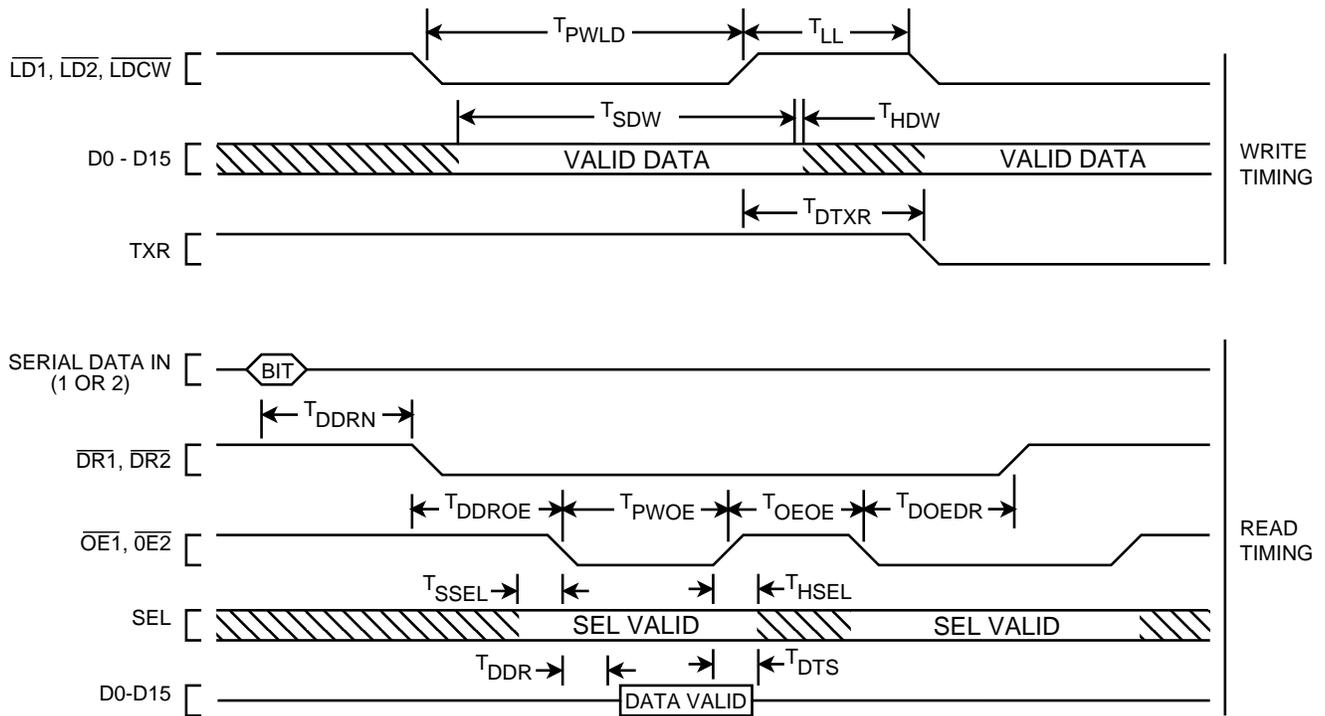
FIGURE 6. READ/WRITE TIMING
