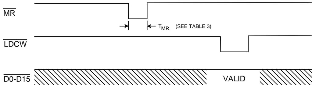
**FIGURE 5. RESET AND INITIALIZATION SEQUENCE**
